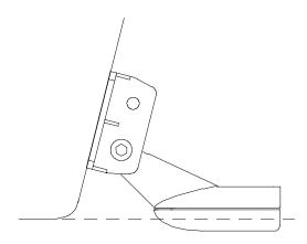
Mark the transom in the center of each slot in the transducer bracket. Now drill one hole in the center of each slot. Use #12 stainless steel screws (not included) to loosely attach the brackets to the transom.
